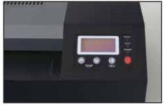
3. Use the guide located on the front of the machine to select proper temperature and speed. Wait for ready light to turn solid green & machine beeps.
