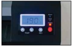
6. To turn off, reduce temperature to 190°F and wait approx. 15 min. Press the Power Button twice then switch off the Power Switch in the back.
