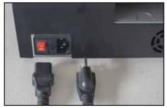
1. Use the female connector of the power cord to plug into the back of the machine. Use the male connector to plug into an appropriate power source.
